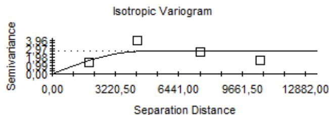
Spherical model ( $C_0 = 0,0010$ ;  $C_0 + C = 2,6410$ ;  $A_0 = 4480,00$ ;  $r_2 = 0,327$ ;  $RSS = 2,97$ )
