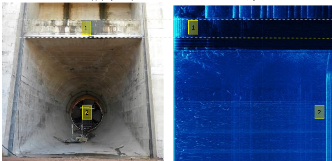
Figure 3 – Jirau HPP draft tube (left). Image capture of the confined ichthyofauna movement in the draft tube after applying the hydraulic flow rate increase maneuver (right).
