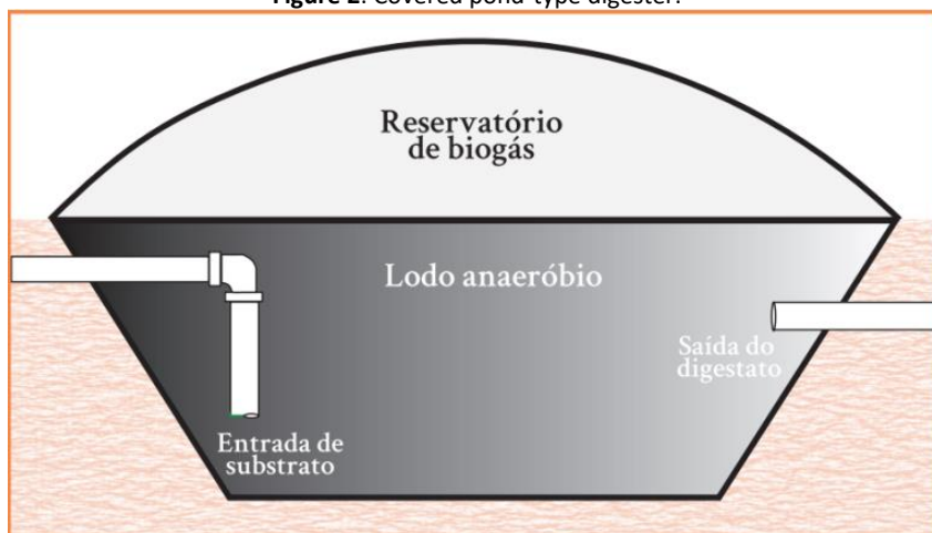
Figure 2: Covered pond-type digester.
