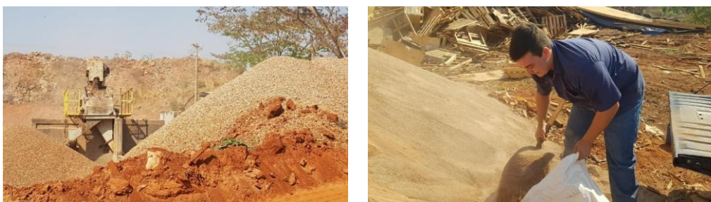
Figure 1: The image on the left is from Mejan Ambiental's recycling material processing and on the right, collection of recycled sand - R-CCW, Votuporanga/SP, 2020.
