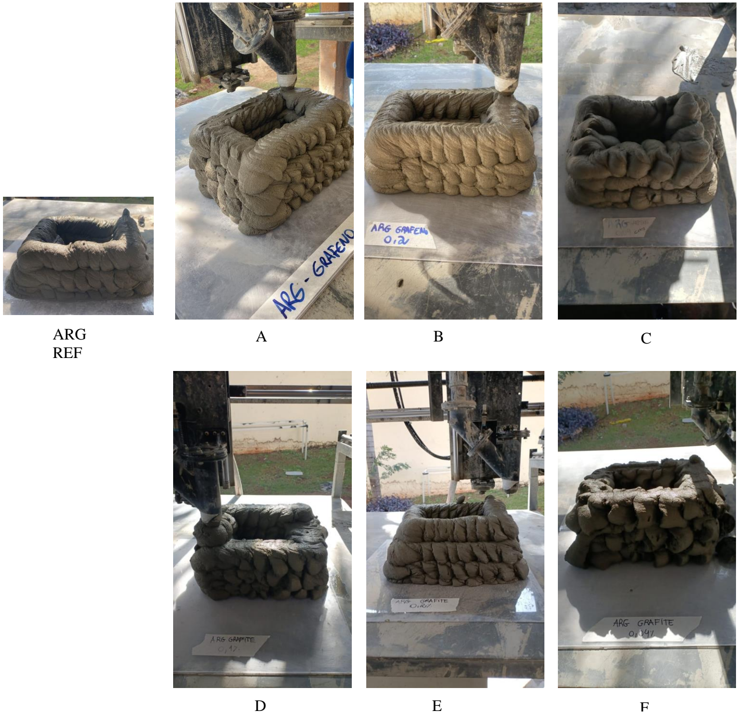
Figure 4 - Images of the constructability test
