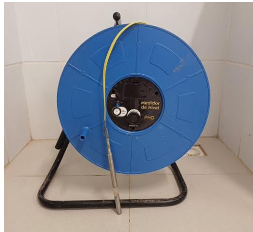
Figure 3 - Electronic piezometric level sensor.
