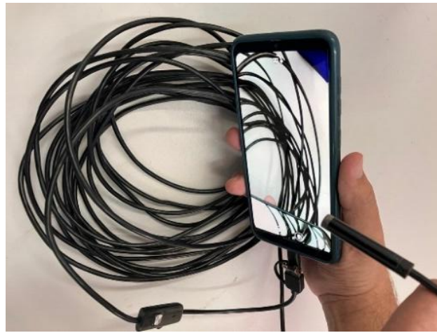
Figure 4 – Video borescope camera.
