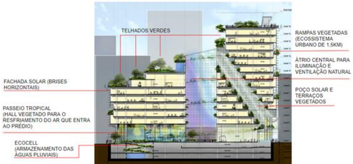
Figure 5 - Schematic section indicating the main bioclimatic strategies used by architect Ken Yeang.
