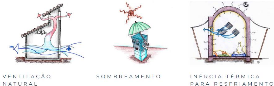
Figure 2 – Main bioclimatic strategies recommended for the city of Belém (PA), also applicable to Singapore.
