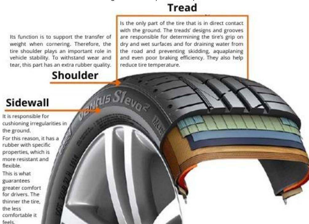
Figure 2 – Description of tire parts
