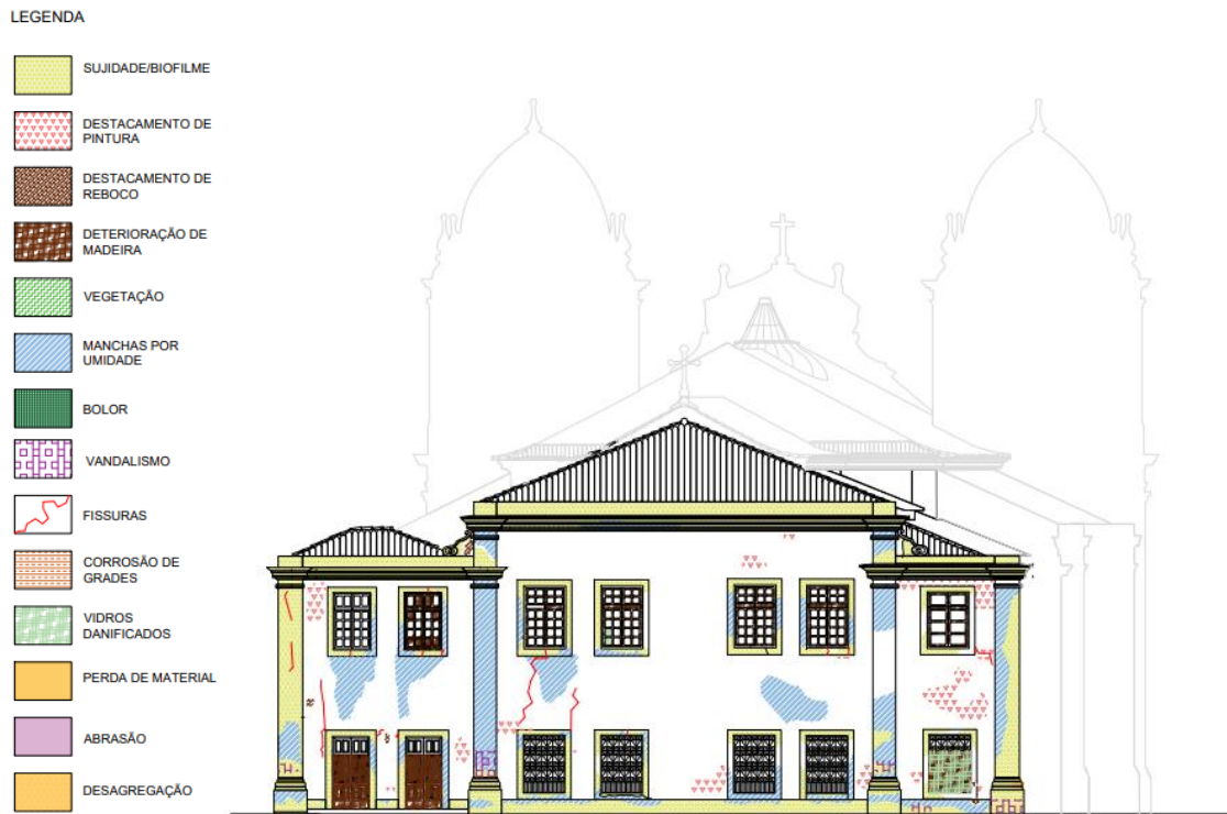
Figure 5 - Damage Map of the West Facade of the Madre de Deus Church
