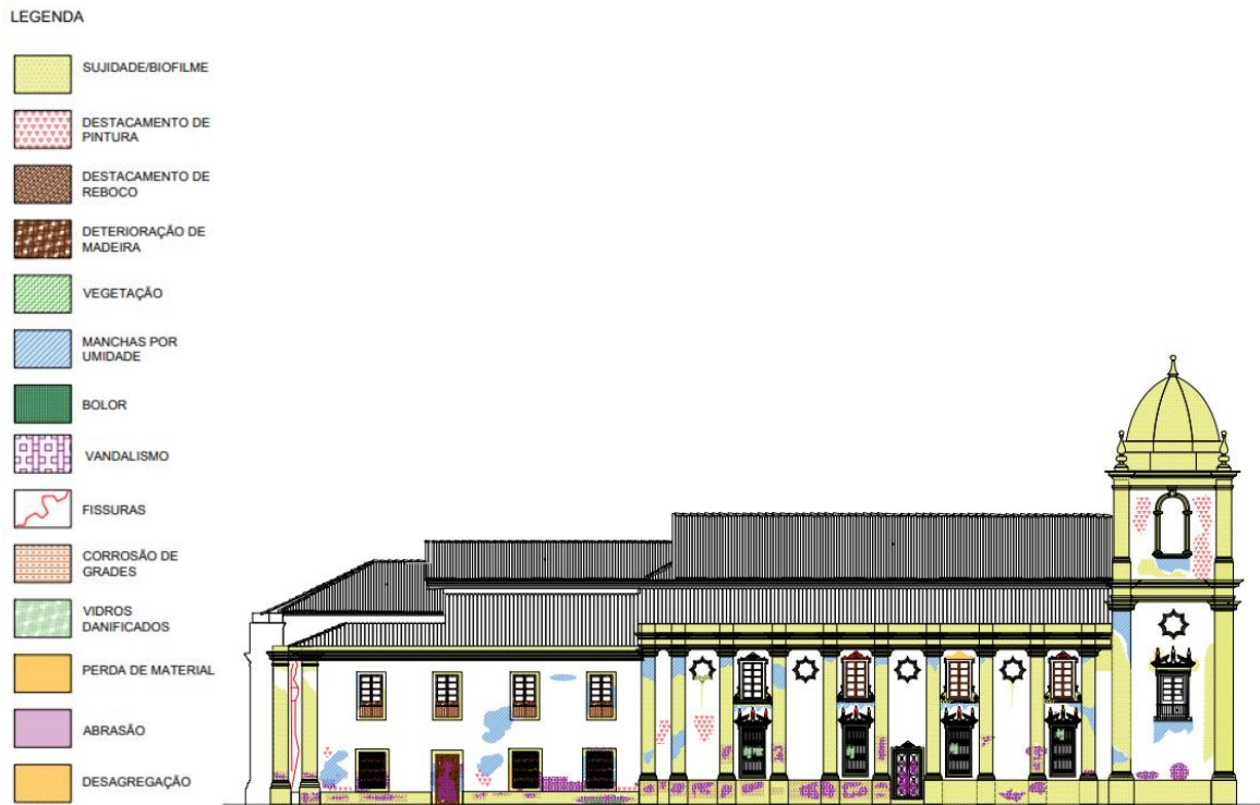
Figure 3 - Damage Map of the South Façade of the Church of Madre de Deus
