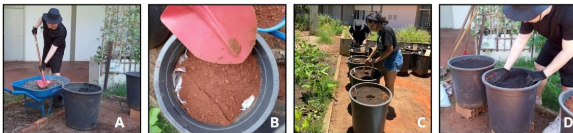
Figure 4 – Experiment setup. A - Placement of the basalt gravel layer. B - Addition of cerrado soil over the geotextile fabric (bidim). C - Sowing of the species. D - Application of a thin layer of topsoil.
