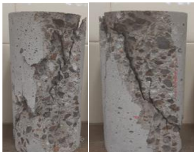
Figure 7: a) Type D - Conical and Sheared and b) Type E - Sheared
