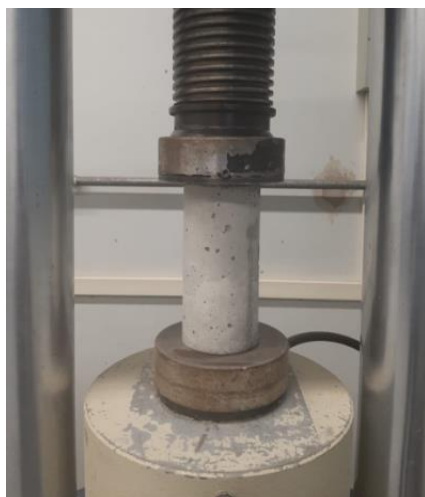
Figure 6: Compressive strength test
