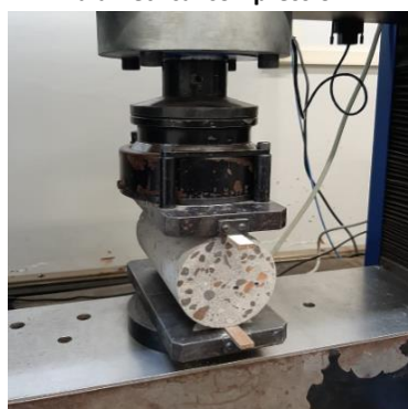
Figure 3: Tensile strength test by diametrical compression
