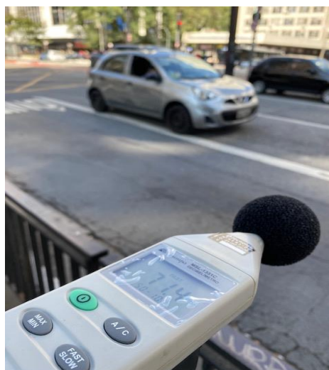
Figure 4: Device - Minipa MSL-1351 C - Decibel meter - capturing the sound pressure level Db.
