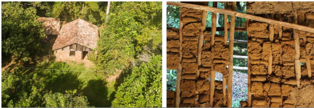
Figura 4 – Flour Mill and constructive technique of wattle and daub
