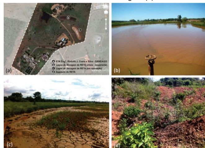
Figure 2: Satellite image of the WTPR area (a); Drying lagoon in operation (b); Full drying lagoon (c); Waste disposal in an area next to the lagoon (d).
