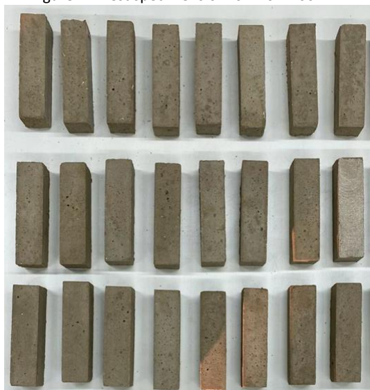
Figure 2 – Test specimens of 40 x 40 x 160 mm
