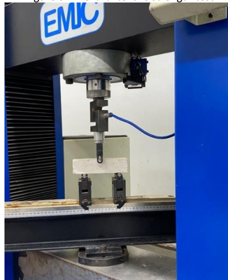
Figure 3 – Flexural tensile strength test
