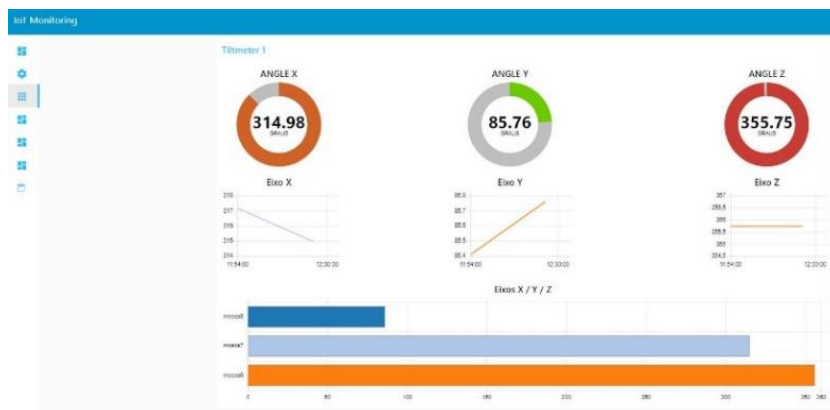
Figure 5 - Angles view screen received in Node-RED
