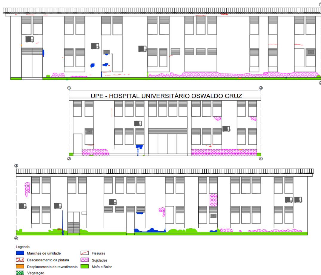
Figure 5 - Damage Map of the Southeast Facade
