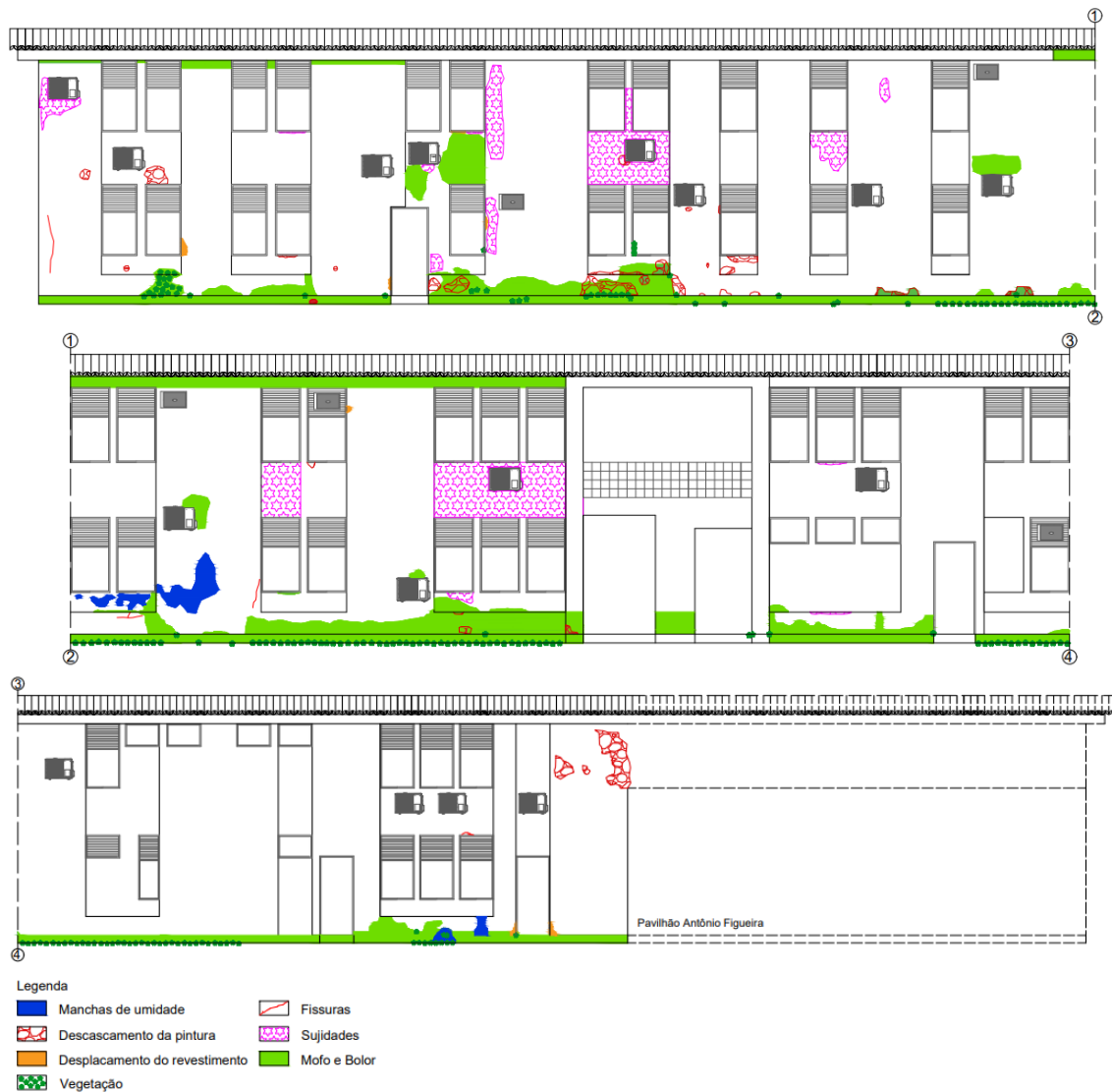
Figure 7- Damage Map of the Northeast Facade
