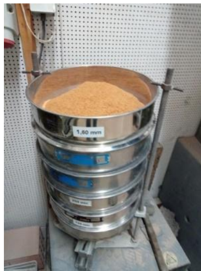
Figure 2 – Checking the grain size
