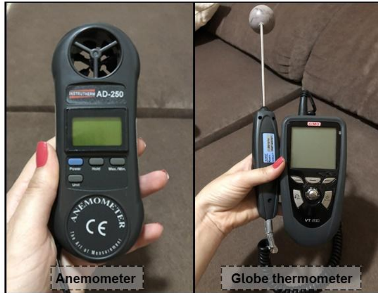
Figure 6- Measuring equipment used in the field.
