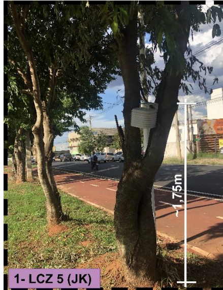
Figure 4- Positioning of the measurement equipment in the field.
