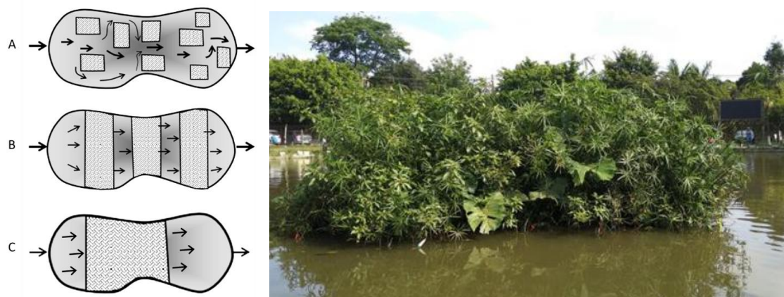
Figure 1 – Design options for FTW positioning and hydraulic flow simulation (left). Photograph of the implemented project (right).
