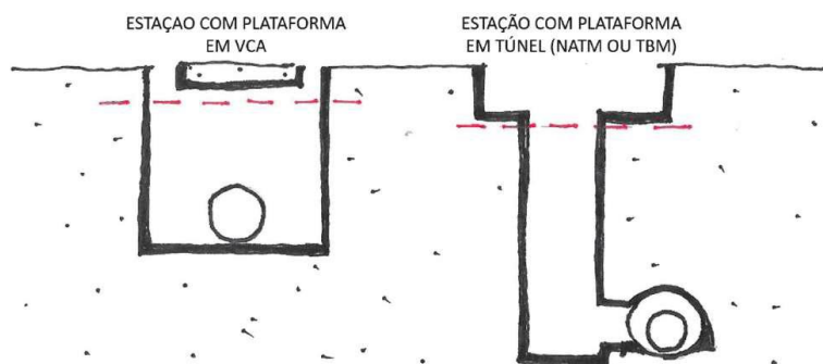
Figure 2 – Sketch of typical cross-sections of shallow standardized stations (in VCA) and deep stations (with platform in conventional NATM tunnel 3 ), with a red dashed line representing the boundary between the standardized deep section and the surface customization.
