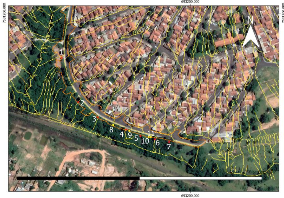
Figure 11: Flow concentration lines and locations of erosion.
