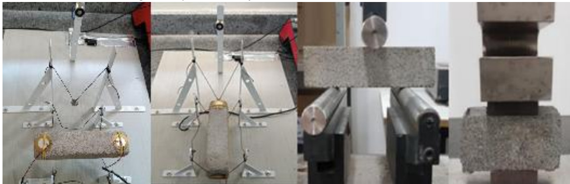
Figure 1: Specimens subjected to acoustic and mechanical tests.
