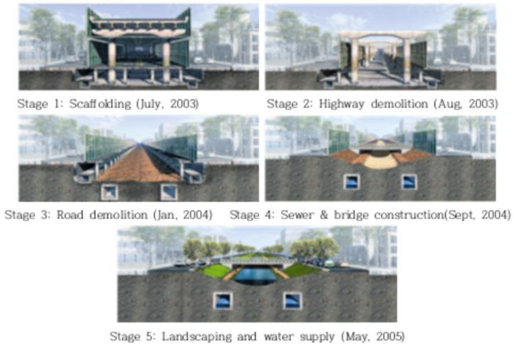
<Figure 13> Stages of the Cheonggyecheon restoration work
